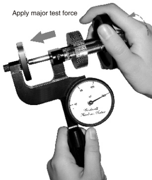
Fig. 9 Apply major test force
